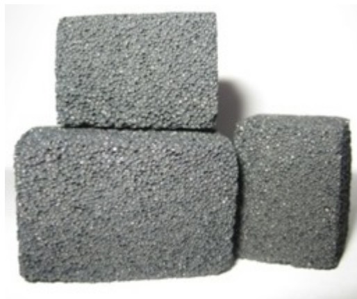
Figure 2. Photo of samples of porous glass composite obtained by low-temperature technology
